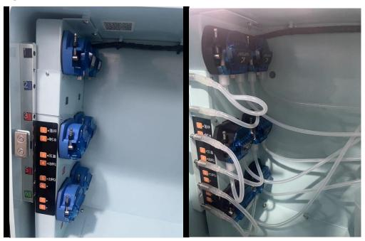
6 peristaltic pumps are controlled by control board in syrup box through RS485.
